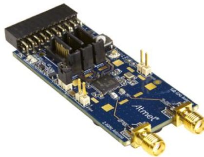
Figure 2.7 The ATREB215-XPRO-A evaluation board, integrating the AT86RF215 transceiver and all necessary support circuitry.
