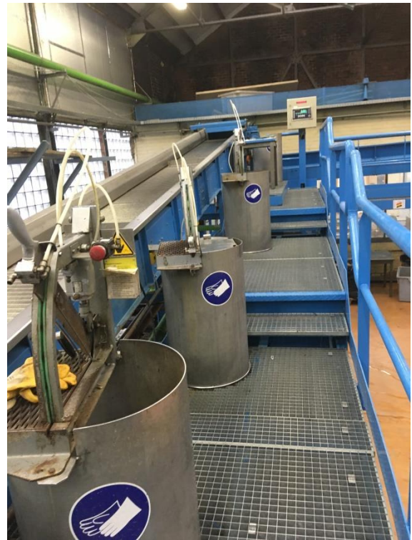
Figure 23: Table de tri des betteraves.
