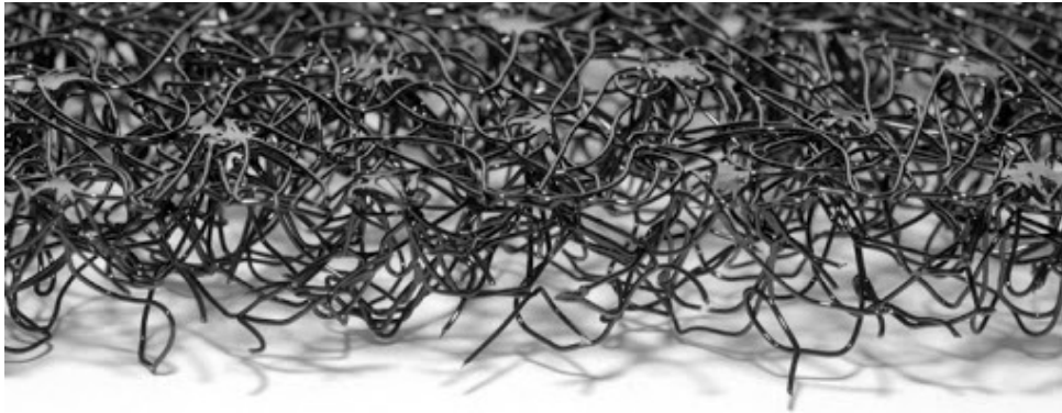
FIGURE 4.13 – Substrat de type géotextile, Enkamat (Geo-Synthetic, nd).
