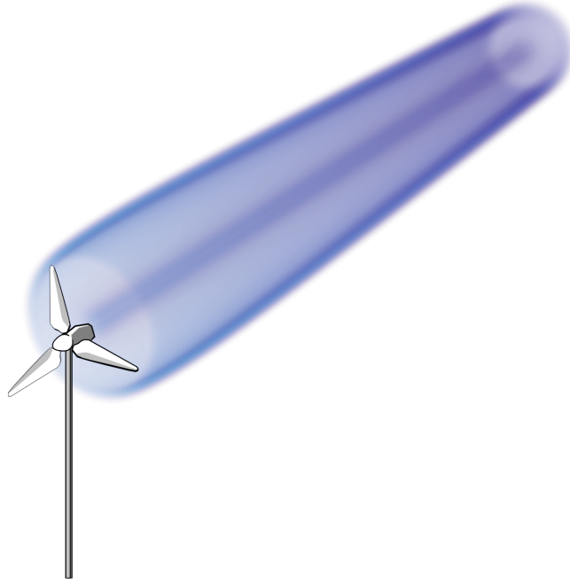
Figure 4.3: Volume rendering of the vorticity field for a baseline-controlled wind turbine.
