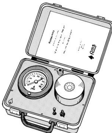
Figure 5: A commercially available pressure chamber. The pressure chamber is designed for either laboratory or field use. A safety valve on the lug cover ensures that pressure can be applied to the chamber only when the cover is properly and completely secured.
