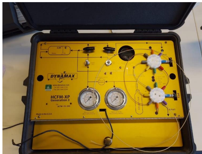
Figure 6: The Hydraulic Conductance Flow Meter.
