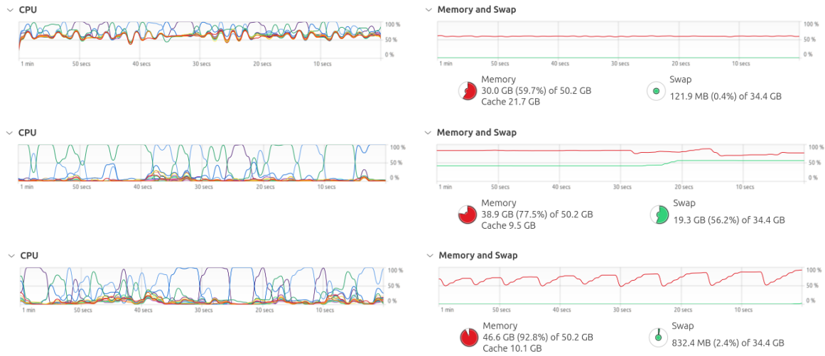
Figure 1.1: Performance regimes, top to bottom: (1) frangi inference, (2) single core ops, (3) sawtooth RAM use
