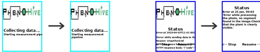
Figure 3.12: Improved display: in "Collecting data" with a line break (left) and in "Status" with date formatting plus a line break (right)
