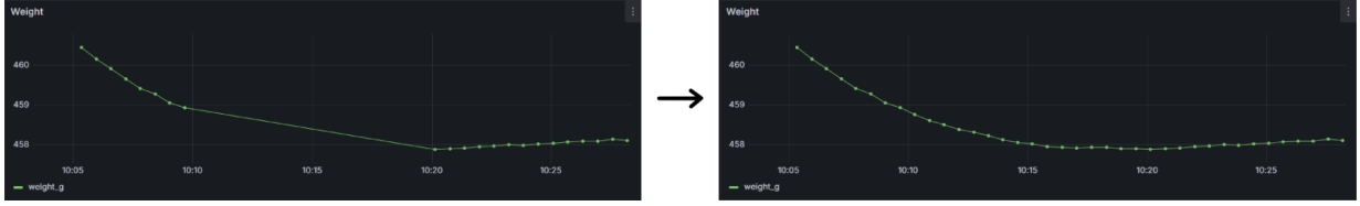
Figure 6.3: Difference between measurements without (left) and with (right) the data recovery system
