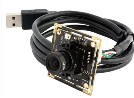
Figure 2.2: ELP AR0330 camera module used for visual acquisition. Adapted from [1].
