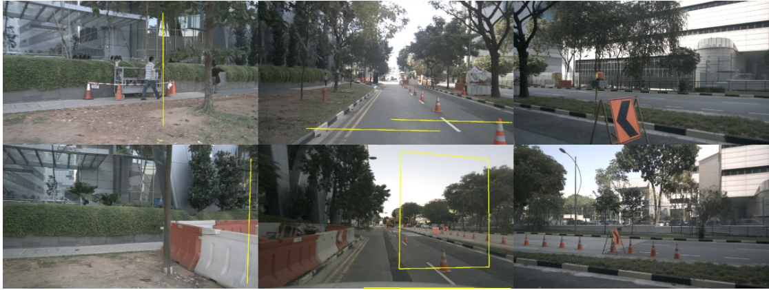
Figure 5.3: Qualitative visualization of the radar-only predictions produced by RCBEVDet. The six camera views are displayed together with the projected bounding boxes obtained when only radar information is used at inference time. Although detections are produced, the predicted bounding boxes are clearly mislocalized which is consistent with the null quantitative results reported in Table 5.7.
