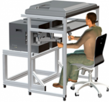
Figure 3.1: Kinarm end-point robotic device: Experimental setup used to collect behavioral data. Participants sat in an adjustable chair and gripped the handle of the robotic arm with their right hand. The device acquires the X and Y positions of the handle in real-time.
