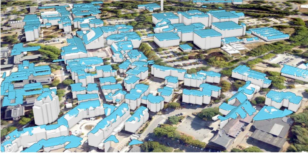
Figure 13 LoD2 Model Obtained by Semi-Automated Modelling overlaid with 'Building' LiDAR point cloud
