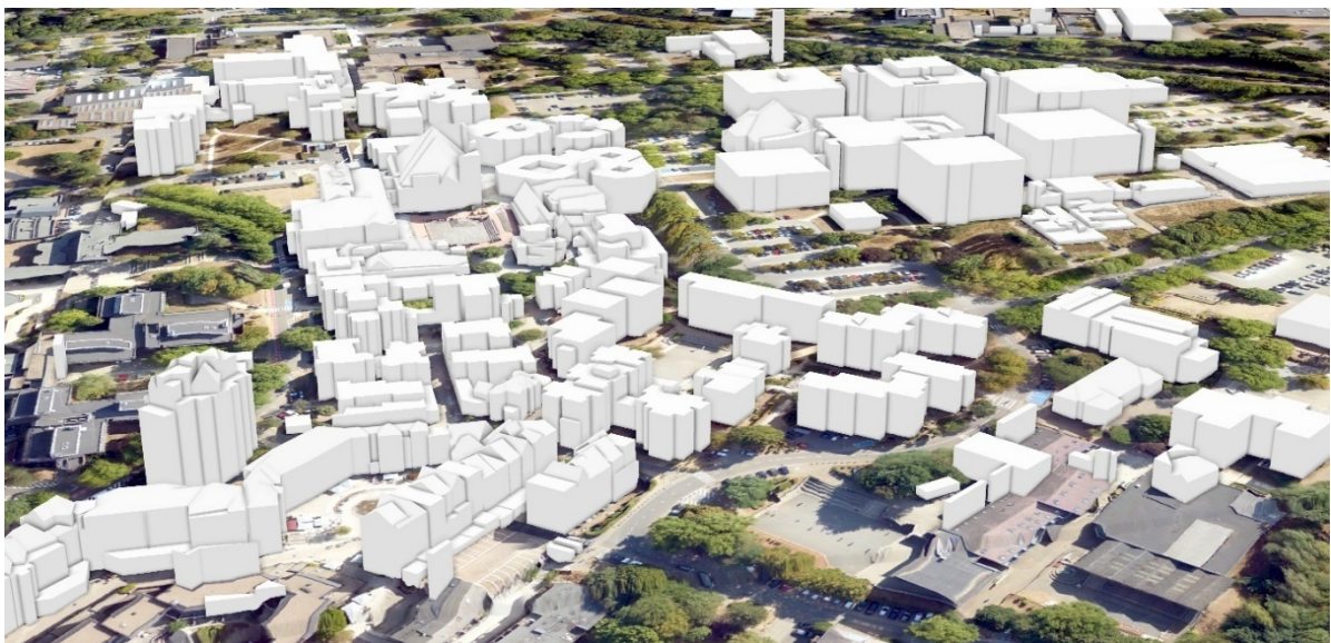
Figure 12 LoD2 Model Obtained by Semi-Automated Modelling
