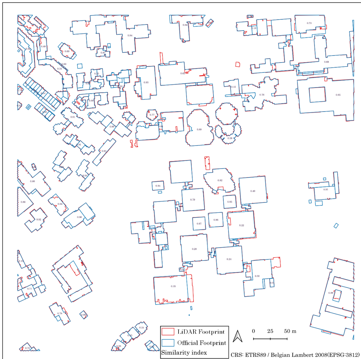
Figure 22 LiDAR derived footprints and PICC footprints with their similarity indices
