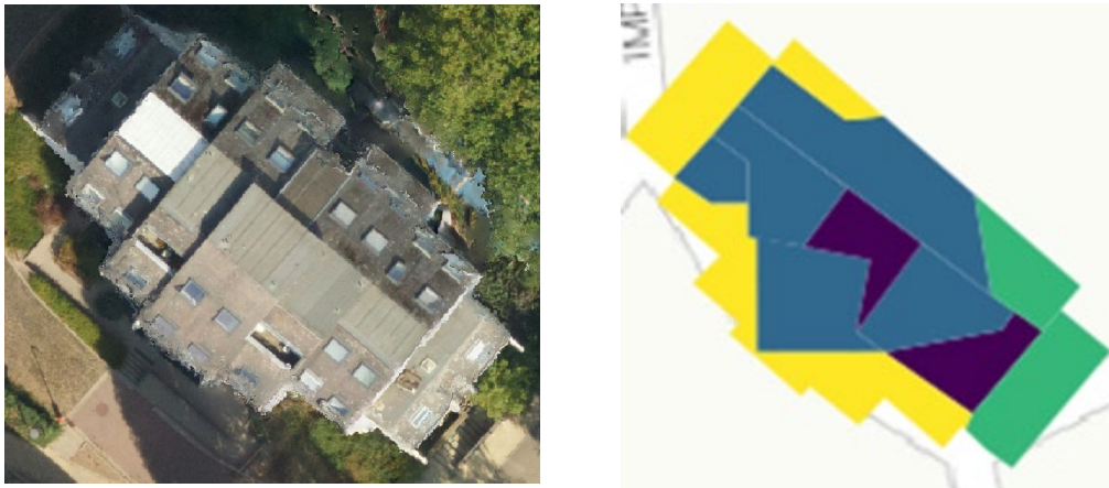
Figure 33 left: Building A4 in orthophoto; right: RMSE class of A4 building (yellow represents the highest value, followed by green, blue, purple)
