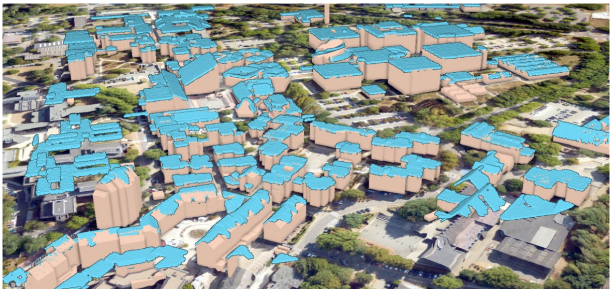
Figure 21 Adjusted LoD2 Model overlaid with 'Building' LiDAR point cloud
