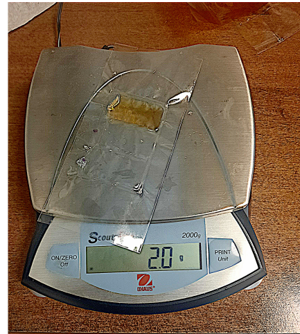
Figure 22: Different steps of filling a pouch (A) Weighing the unfilled HASEL. (B) Inserting the syringe's needle in the pouch through the filling port and clamping the port. (C) Filling the pouch. Rassembling the air bubbles into one (circled in red) and sucking it out. Filling the rest of the oil (D) Pouch filled. Removing the syringe. (E) Sealing the filling port with the soldering iron. (F) Weighing to check the volume filled. Repeating all the steps for all the pouches.
