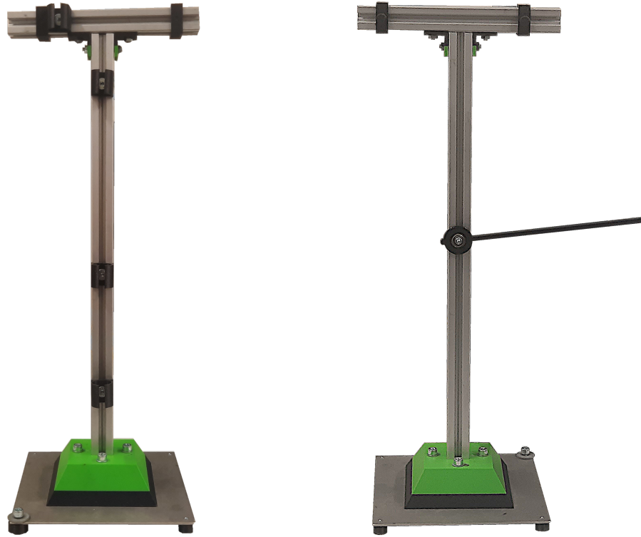
Figure 31: Demonstrator's mount. On the left, the backside shows the guiding pieces for the cables. The bigger screw with the washer are on the left bottom corner. On the right, the frontside shows the pulley with its arm lifted. Attachments pieces are on the horizontal profile at the top. The brackets and the 3D-printed base that join the profiles and the plate are in black and green. Screws with nuts clamp the mount together.
