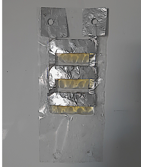
Figure 24: Types of electrodes tested. (A) Canvas for graphite spray paint. We observe that the paint has a laquered aspect showing that it takes a liquid form. (B) Spray-painted electrodes. Its delimitations are not clean. We can also see traces laid when handling the HASEL. In fact, the paint does not adhere well to the plastic sheet. (C) Graphite liquid paint electrodes. We use the same type of canvas with tape for the electrode's shape. Delimitations are more clear but still vague. The liquid paint adheres a bit better than the spray but still comes off easily. We still have traces of graphite on the rest of the sheet. (D) Aluminium electrodes. The electrode's shape is cut before the positioning using a cardboard canvas. The delimitations are clear.
