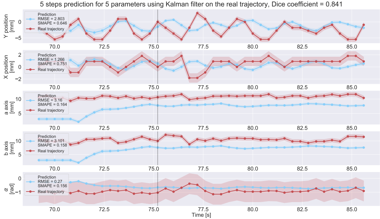
Figure 5.27: 5 steps prediction for 5 parameters using Kalman filter on the real trajectory. The mean real trajectory in red, the measurements in light red and the prediction in blue. The model is found with a system identification using N4SID/MOESP. P1C. Testing set. 100 simulations.
