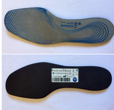
Figure 3.2: Instrumented Insole, Feetme One
