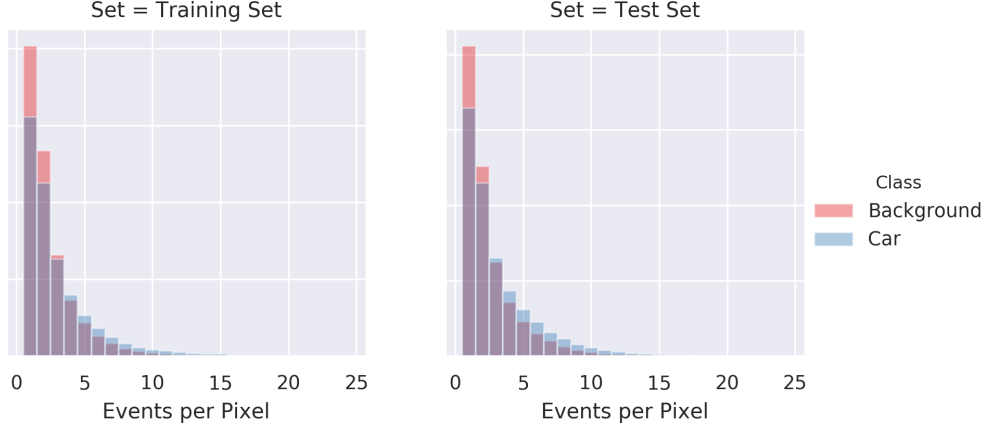
Figure 3.7: Distributions of the number of events in a sample for a single pixel in the 1K subset of N-CARS.
