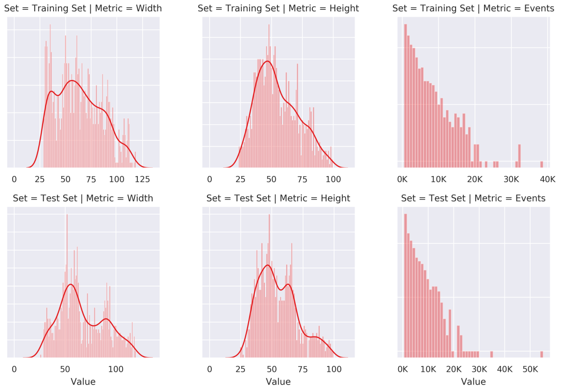
Figure 3.4: Distributions of the width, height and number of events in the 1K subset of N-CARS.
