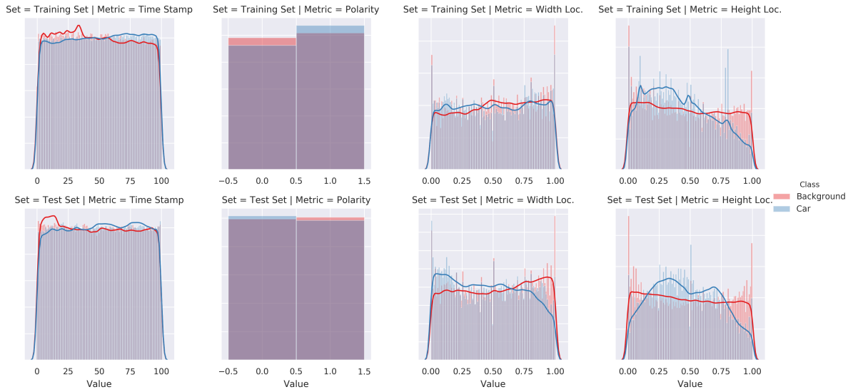
Figure 3.6: Distributions of the time stamps, polarity and location of the events in the 1K subset of N-CARS.
