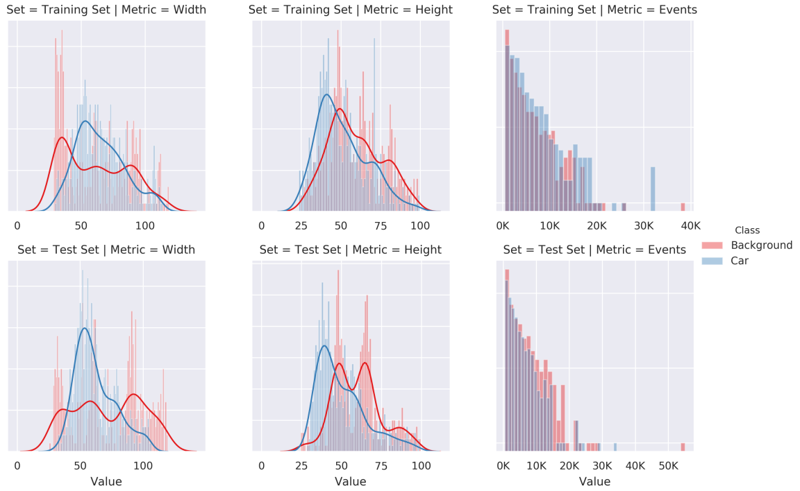
Figure 3.3: Distribution for the width, height and number of events for each class in the 1K subset of N-CARS.
