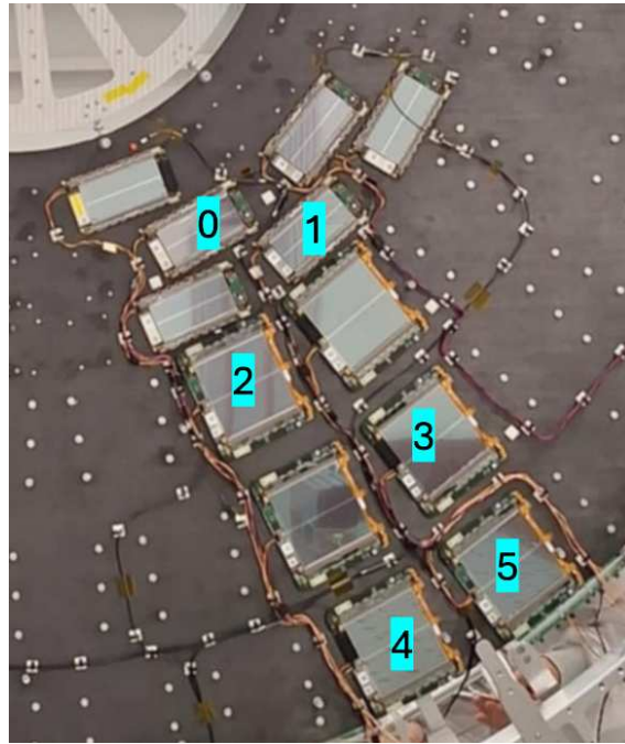
Figure 7.1: Zoomed-in view of figure 5.1 with a label on the working modules on the dee. Modules 0 and 1 are PS modules, and the four others with labels are 2S modules.
