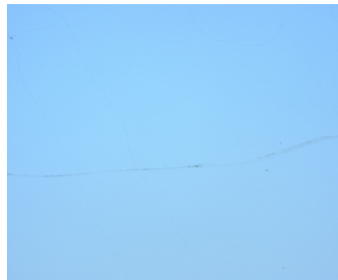
(b) Cracks on the middle of the wafer.
