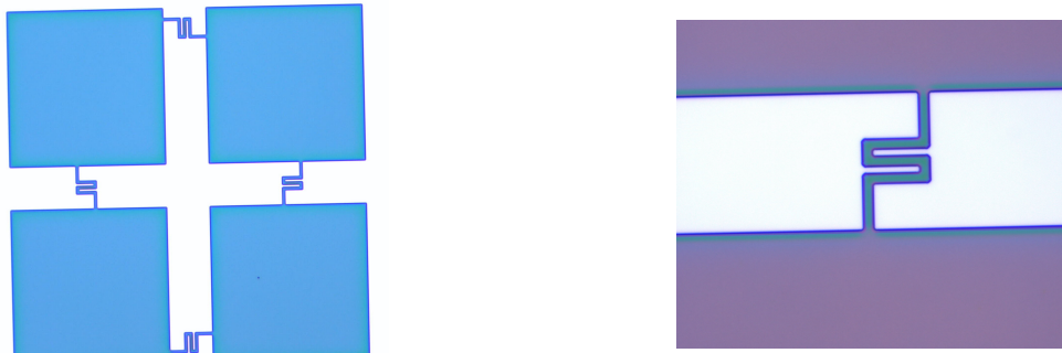
(b) Resolution of the piezoresistor.
