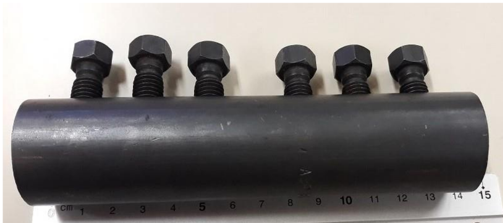
Figure 8 Mechanical coupler used to connect the SMA and the standard steel rebars in the test unit RC+SMA (T. Herrezeel, 2019)
