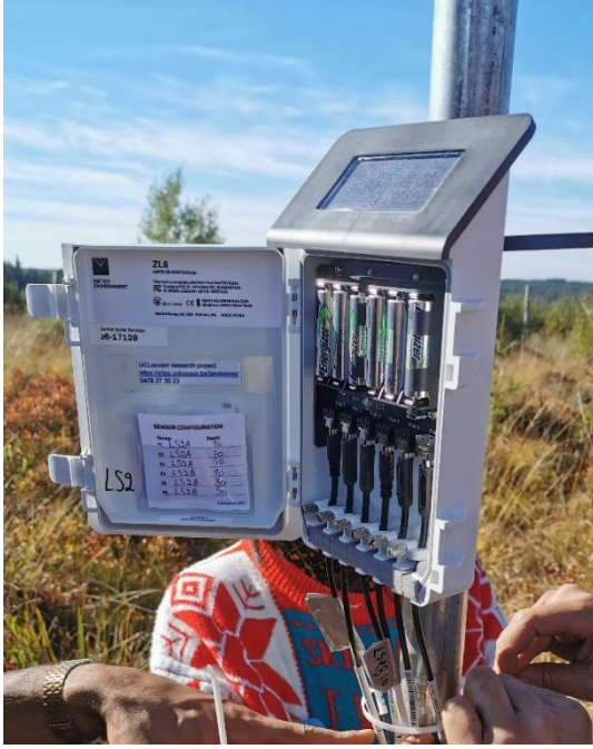
Figure 26: ZL6 Data logger connected to the probes.
