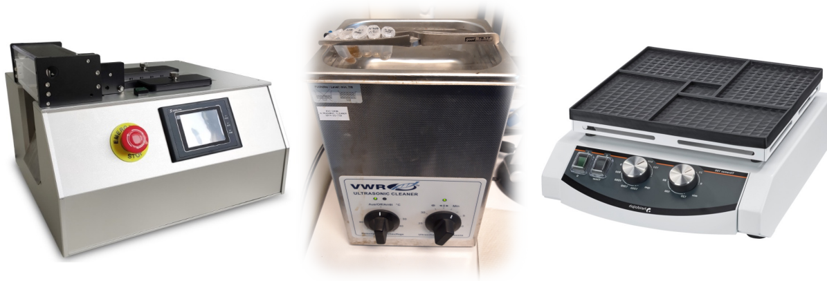
Figure 4.8: Some equipment used, Left: Strip cutter (image from KjnBi manufacturer), Middle: ultrasonic bath, Right: shaker (image from Heidolph manufacturer)
