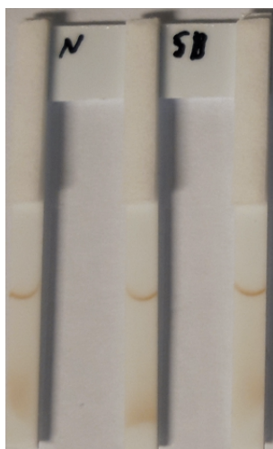
Figure 5.7: Left: Control line with MNP@Neutravidine in running buffer Right: Peak depth obtained with different running buffer. RB:initial running buffer, T20:Tween 20. As we can see running buffer composed of only BSA and Tween 20 2% did not enable the appearance of a control line.
