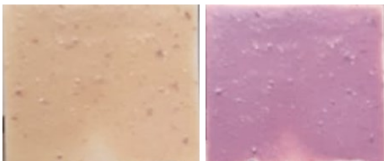
Figure 40 PU- [\text{Fe}(\text{NH}_2\text{trz})_3]\text{Br}_2 \cdot n\text{H}_2\text{O} Hybrid obtained via In situ synthesis. (left) HS state (right) LS state
