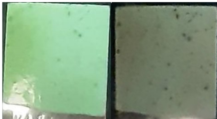
Figure 91 Fluorescent coating in the HS state (left) and in the LS state (right)
