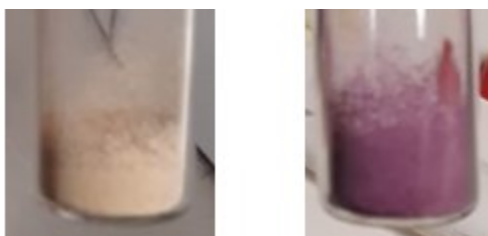
Figure 37 [\text{Fe}(\text{NH}_2\text{trz})_3]\text{Br}_2 \cdot n\text{H}_2\text{O} at room temperature, synthesized via mechanochemical synthesis, in the HS state (left) and LS state (right)
