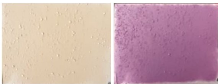
Figure 48 Thermochromic properties of the first hybrid coating tests. Coating at room temperature in the HS state (left) and LS state (right)
