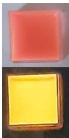
Figure 97 Rhodamine derivative fluorescent polymer Up) under visible light Down) under UV light
