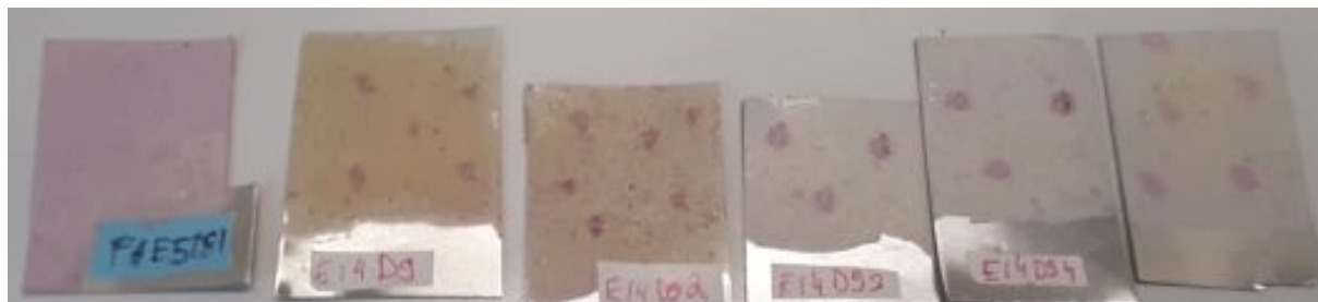
Figure 58 Comparison of thermochromic properties of [\text{Fe}(\text{NH}_2\text{trz})_3]\text{Br}_2 \cdot n\text{H}_2\text{O} coatings -DMPA in the SCO synthesis (coating 1 from left to right), +DMPA into synthesis (coatings 2-3), +DMPA + \text{TiO}_2 (coatings 4-6). Purple dots demonstrate the piezochromism of these compounds. Coating 1 has a thinner hysteresis and partially reverts to the LS state (purple) at room temperature.
