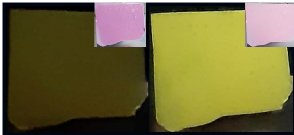
Figure 97 Rhodamine derivative fluorescent polymer Up) under visible light Down) under UV light
