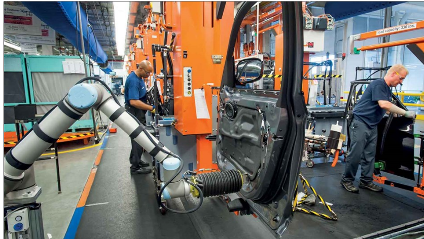
Figure 1.1: A UR5 from Universal Robotics used as a collaborative robot on production lines in a car factory (reference: Picture link ).
