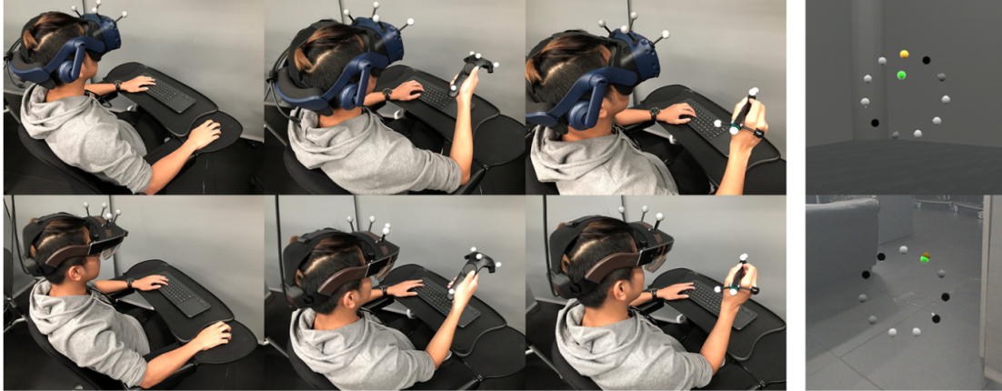
Figure 2.10: Experimental setup to evaluate pointing performances of several devices, from [15].
