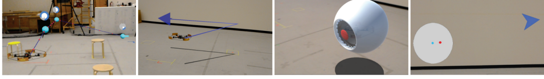
Figure 2.4: 4 different AR-based visual effects to improve human-robot collaboration in the case of an aerial robot, proposed by the paper [8].
