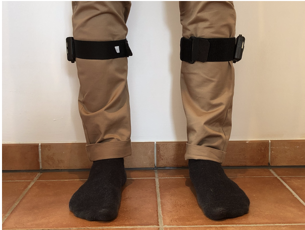
Figure 5.3: Experiment #1 : IMUs on the lateral side of the left and right tibias.
