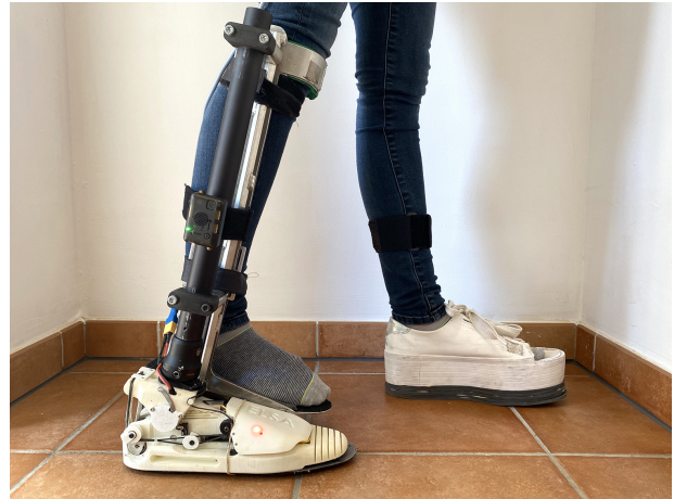
Figure 5.4: Experiment #2 : ELSA active ankle prosthesis during an overground walking experiment performed by an able-bodied subject wearing an adapter.
