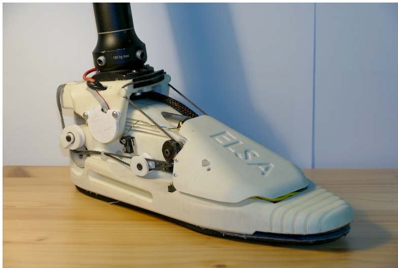
Figure 2.9: Prototype of the ELSA prosthesis made by F. Heremans.
