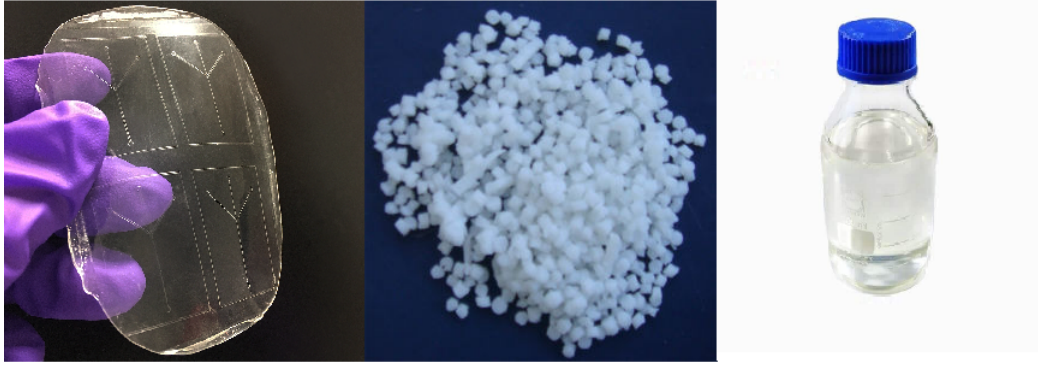
Figure 3.3: Necessary materials for the fabrication of a transfer blade. PDMS, PPC, and PPC diluted in anisole in a. and b. and c. respectively.[25]
