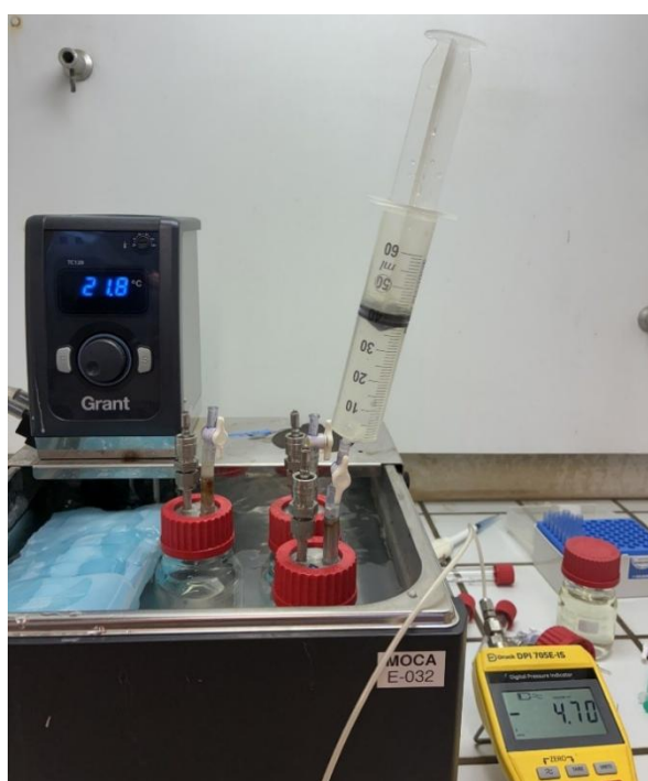
Figure 15 - Air injection using a 100 mL syringe to restore zero pressure by expelling residual water from the connectors.
