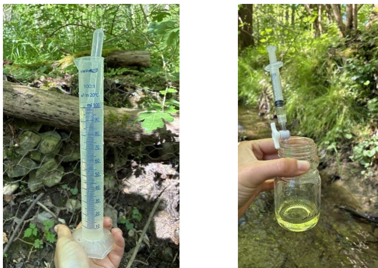
Figure 9 - Photographs of the alkalinity measurement preparation materials. From left to right: graduated cylinder and Pasteur pipette used to collect 100 mL water samples; concentrated acid with syringe and needle used for acid injection.
