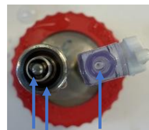
Figure 14 - Zones where water/debris can get stuck
