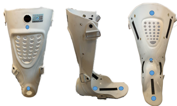
Figure 4.3: Final rigid support (without the drillings) that will fit at the front of the thigh and knee in the final device. The blue circles represent the location of the M6 holes.
