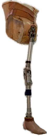
Figure 4.5: Canadian passive left leg prosthesis used to perform stabilization tests on the adapter.
