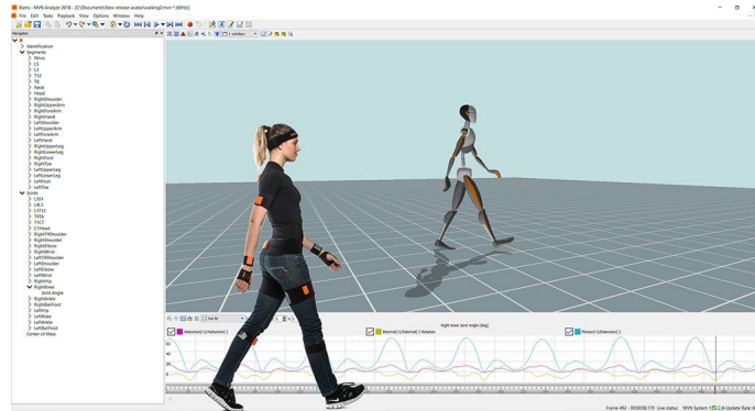
Figure 5.2: Visualisation of the simulation in the MBsysWeb platform interface measured via the XSENS MT sensors.[38]
