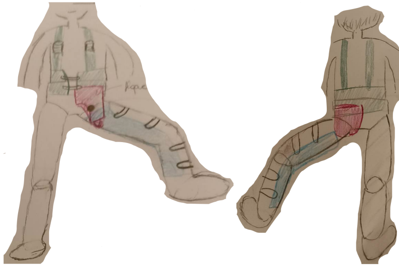
Figure 2.14: Representative sketch of concept 2 without the Canadian prosthesis composed of the corset (green), the gutter (blue) and the piece connecting these two elements (burgundy).
