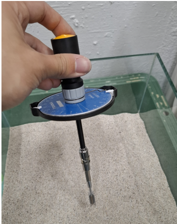
(a) Torque Driver FTD5CN-S used for soil characteristics homogeneity check.
