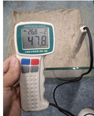
(b) Soil Moisture Meter DM-18R used to assess the homogeneity of saturation level.
