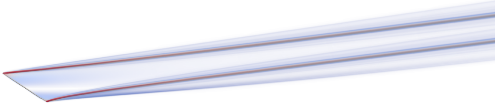
Figure 2.22: Representation of the magnitude of vorticity \zeta in the wake of an elliptical wing solved using the VPM method. (form [33])
