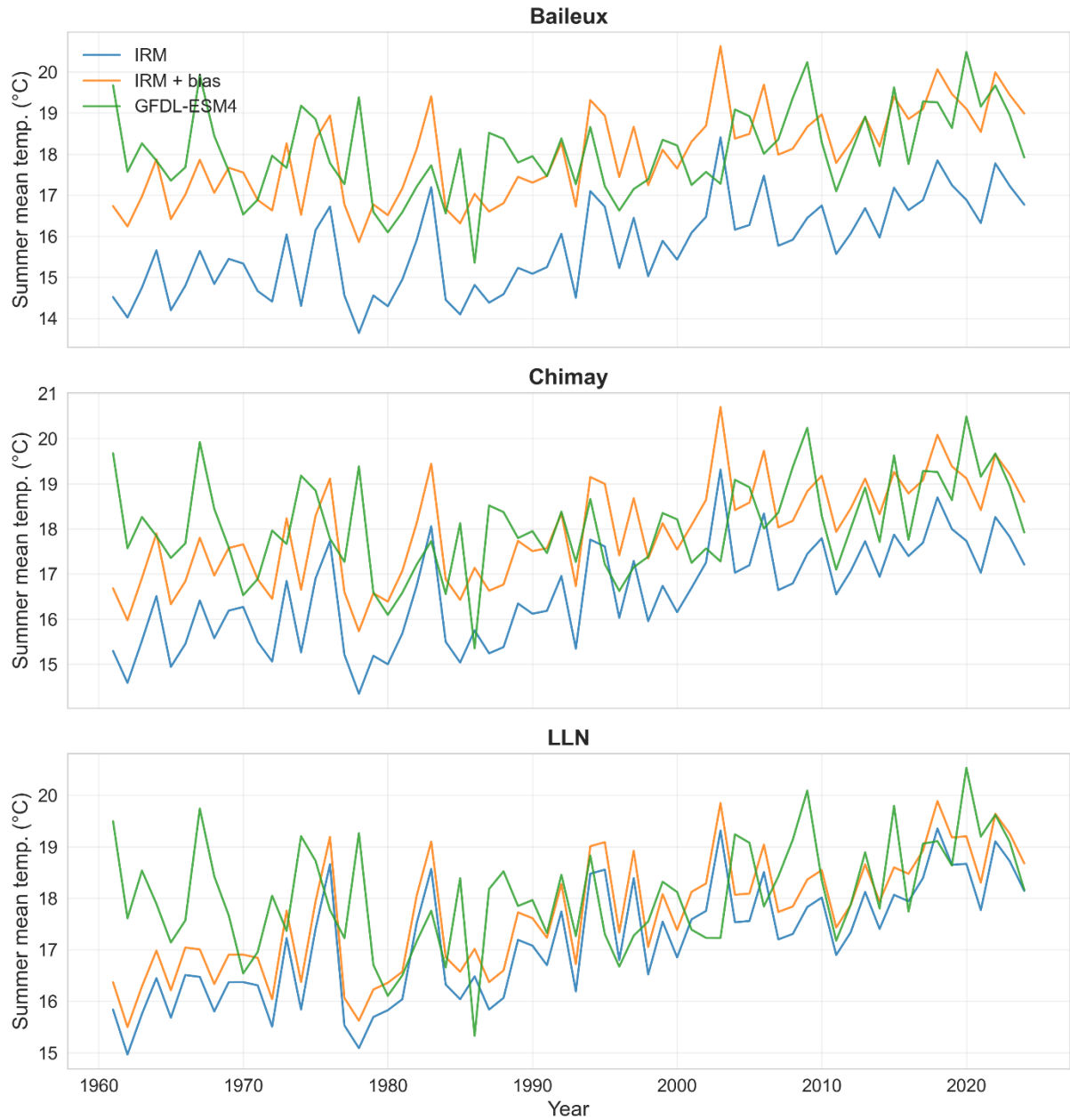
Figure J1 : Summer (June-August) mean temperature time series for the three climate forcings used in the level/residual effect test (section 3.4.3): IRM (observed), IRM+bias (IRM data shifted by a constant offset to reach GFDL-ESM4's mean summer temperature), and GFDL-ESM4, for Baileux, Chimay, and LLN (1961-2024). The close alignment between IRM and IRM+bias confirms that the interannual variability and trend of IRM are preserved in the synthetic dataset, with only the mean level shifted.
