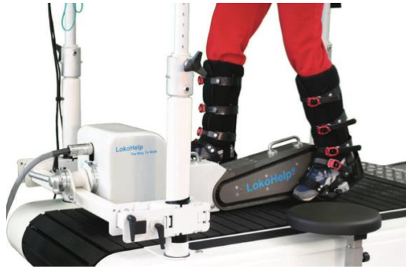
Figure 3 : robot a effecteurs distaux, exemple du LokoHelp 31 ( https://www.mtm.ca/sn_uploads/product/Lokohelp_MTM.pdf )
