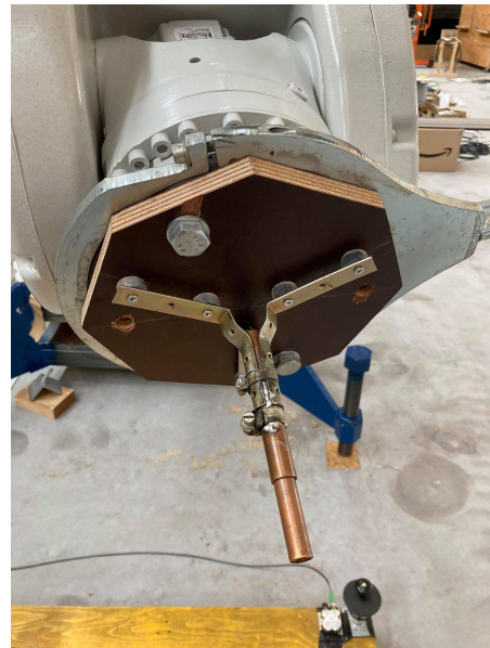
Fig. 4.2: Designed tool to maintain the pen
