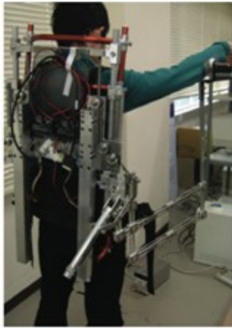
Fig. 1.6: Prototype of aid wearable robot [8]
