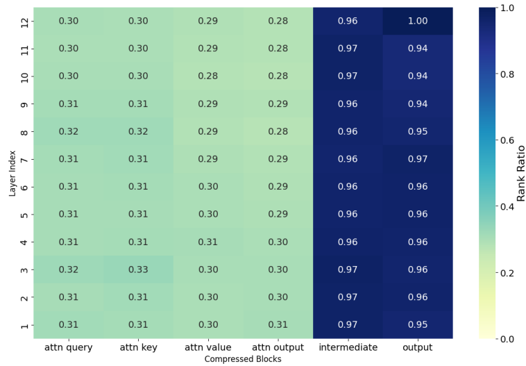
Figure 9: The normalized sorting criteria computed as the ratio between the maximal dimension of a given weight matrix and its effective rank, is shown for the BERT model with K = 72 weight matrices. The first three columns represent, respectively, the query, key, and value weight matrices, with their layer index indicated on the y-axis ranging from 1 to 12. The fourth column corresponds to the attention projection weight matrix, while the last two columns represent the feed forward layers.
