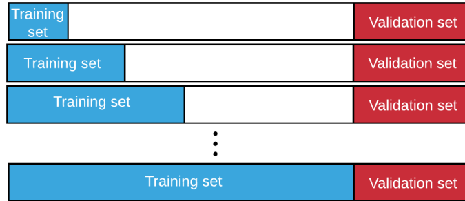
Figure 5.2: To build the learning curves: we build a validation set at the beginning which will remain the same, then, we gradually train the neural network on a training set whose size increases progressively.
