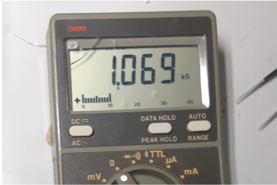
Figure 4.9: Multimeter measurement of the silicon strain gauge.
