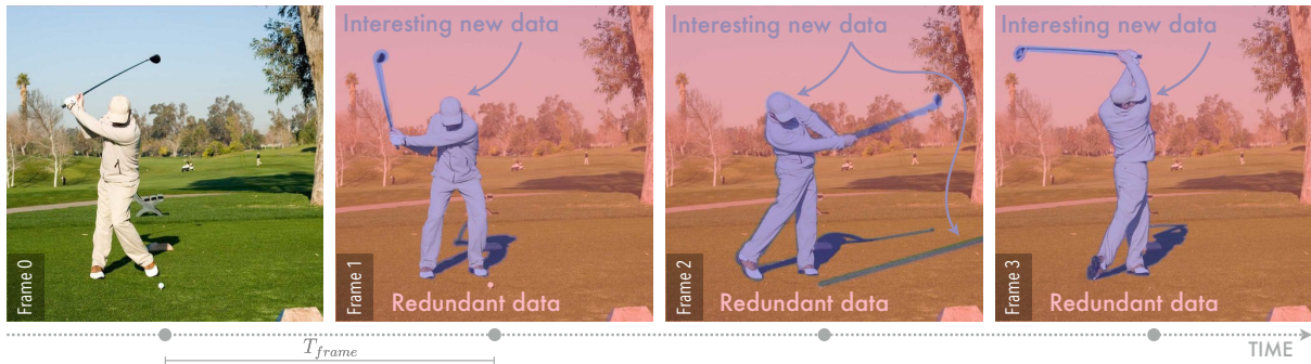
FIGURE 2.1 – Identification of redundant and interesting data in an image obtained with a conventional camera (frame-based sensing). The sky, trees and grass are unnecessary oversampled whereas the swing of the club and the movement of the player/ball are undersampled. Image adapted from [40].
