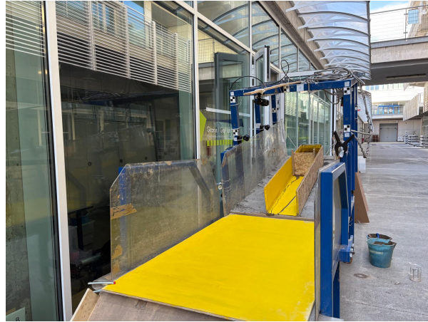
(a) Experimental set-up ready to be used and filled with material. Negligible liquid leakage passes through the gate.
