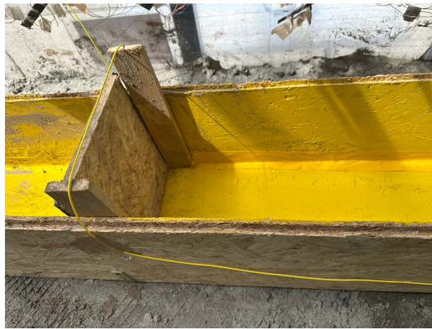
(b) Detail of the inclinable gate and optical fibre used to precisely record the opening time. The material is stored upstream of the gate prior to release.
