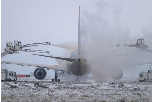
Figure 1.13: B777 on the deicing platform [7]
