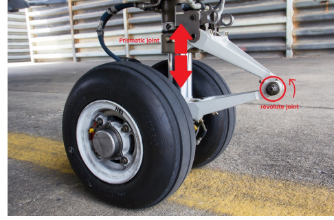
Figure 3.2: The nose wheel suspension joints [19]
