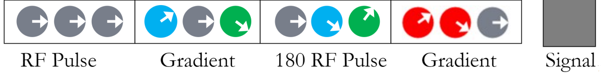
Figure 2.14: Effect of the PGSE sequence on the magnetization without and with diffusion. From [38]
