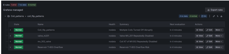
Figure 7.6: Alert rules configured in Grafana based on log patterns
