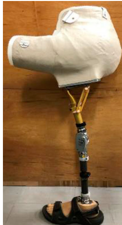
Figure 1.16: Sagittal plane view of the prosthesis designed by Y. Ueyama, mounted on an adapter for able-bodied testing. [23]
