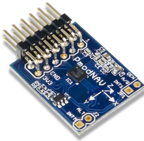
Figure 2.3: PMOD-NAV: 9-axes IMU plus barometer
