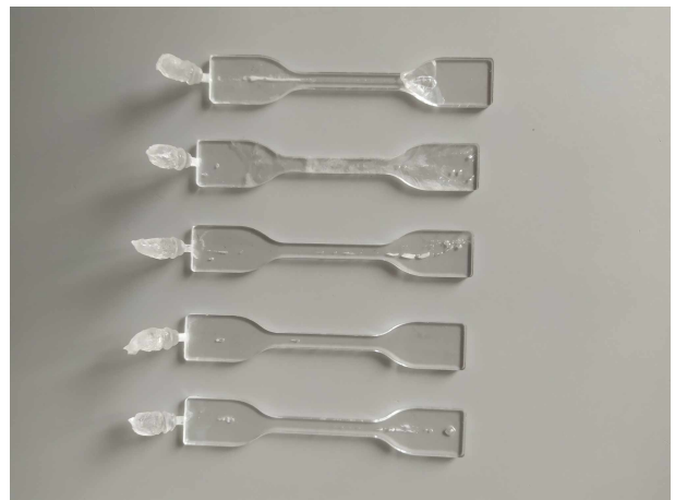
Figure 13: Samples with bubbles.
